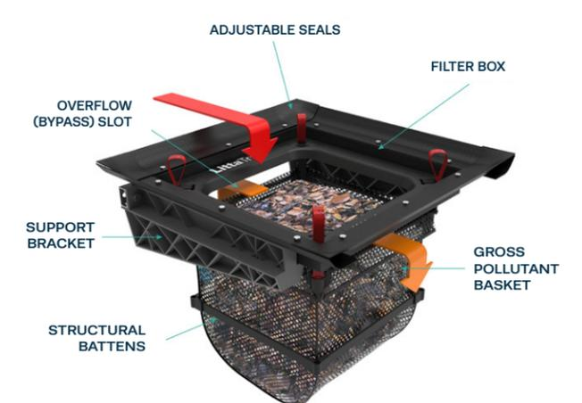
Figure 3: Enviropod® LittaTrap™ FC Bypass Operation
